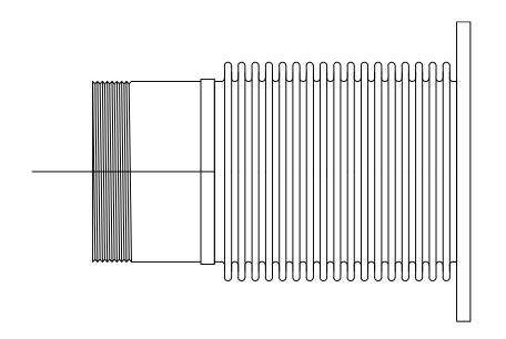
TITLE: SINGLE METAL BELLOW EXHAUST EXPANSION JOINT WITH FIXED FLANGE ONE END AND MALE NPT OTHER END DESCRIPTION: DESIGNED FOR LOW EXHAUST PRESSURE, TEMPERATURE, AXIAL COMPRESSION, LATERAL OFFSET AND ANGULAR DEFLECTION
