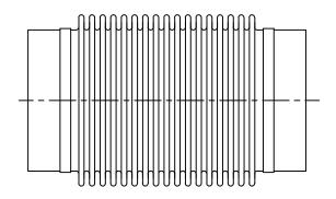
TITLE: SINGLE METAL BELLOW EXHAUST EXPANSION JOINT WITH WELD IN TUBE ENDS DESCRIPTION: DESIGNED FOR LOW EXHAUST PRESSURE, TEMPERATURE, AXIAL COMPRESSION, LATERAL OFFSET AND ANGULAR DEFLECTION
